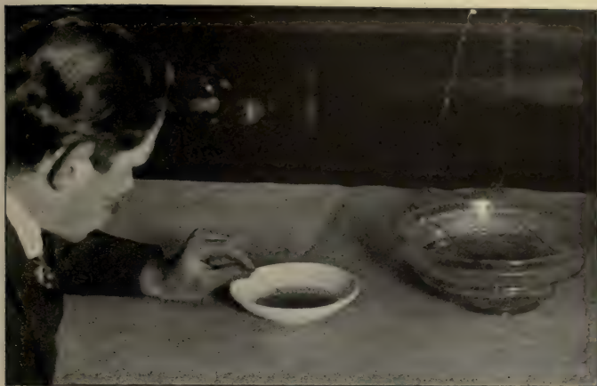
FIG. 177. Cleaning the copper in acids.
